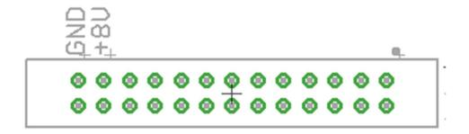
Pin 1 is in the upper right, and it indicated by the small dot. Pin 3 is immediately to its left, pin 5 next, etc. All of the odd numbered pins are in the top row, while the even numbered pins are on the bottom row. Pin 2 is directly under pin 1.
